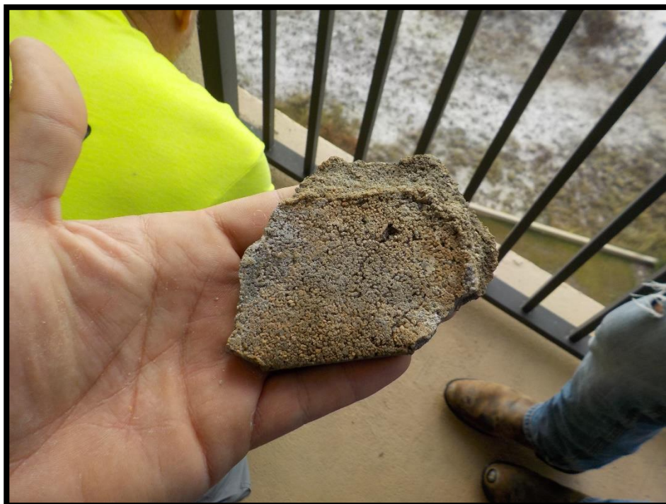
Example of material utilized during “cap” repairs.
